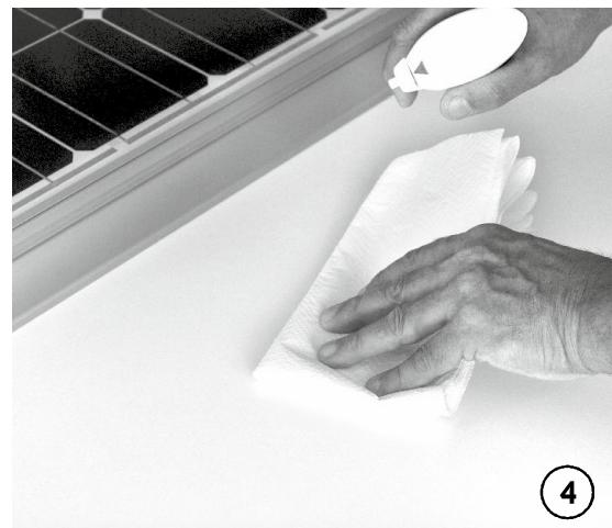
Use a degreasing agent to clean the motorhome roof and glue the spoiler on it. Let the glue dry.
